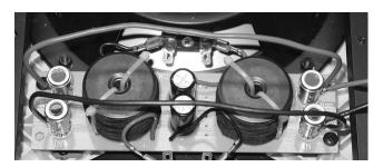
When wiring from a stereo amplifier, connect one set of leads to each set of terminals, observing proper polarity. This will connect each woofer individually as an 8 Ohm load. This is shown in the picture below.
